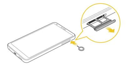
2. Place the Nano SIM card into the correct section of the tray.
