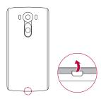
2 Slide the Nano SIM card into the Nano SIM card slot as shown in the figure. Make sure the gold contact area on the card is facing downward.
