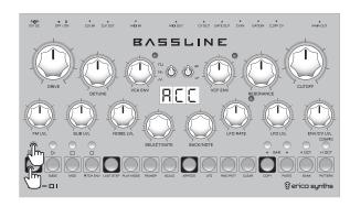
Push and hold the SHIFT button and push the ACC (accent) button! The sequencer will advance to the accent enter mode. You will see 70% dimmed step buttons showing what steps are active in the sequence. Push the step buttons for the steps that you wish to accent, and step button LEDs will go on full brightness. The accent will open the VCA and VCF slightly. To return to the step enter menu, push the BACK/NOTE encoder.
