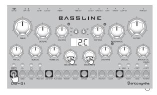
In order to alter the pitch and gate length, push and hold the relevant step button and rotate the NOTE encoder to alter the pitch and the GATE encoder to alter the gate length. The indicator will give visual feedback on settings. 100% gate length means the step is merged with the next one and the envelope will not retrigger.
