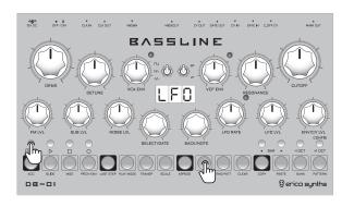
Push and hold the SHIFT button and push the LFO button to access the LFO settings! Rotate the SELECT/GATE encoder to select the function - LFO shape (SHP), synchronized/free running (SYC) LFO or LFO reset on each active step. Rotate the BACK/NOTE encoder to make a selection. The step buttons will give visual feedback of the LFO in action.
