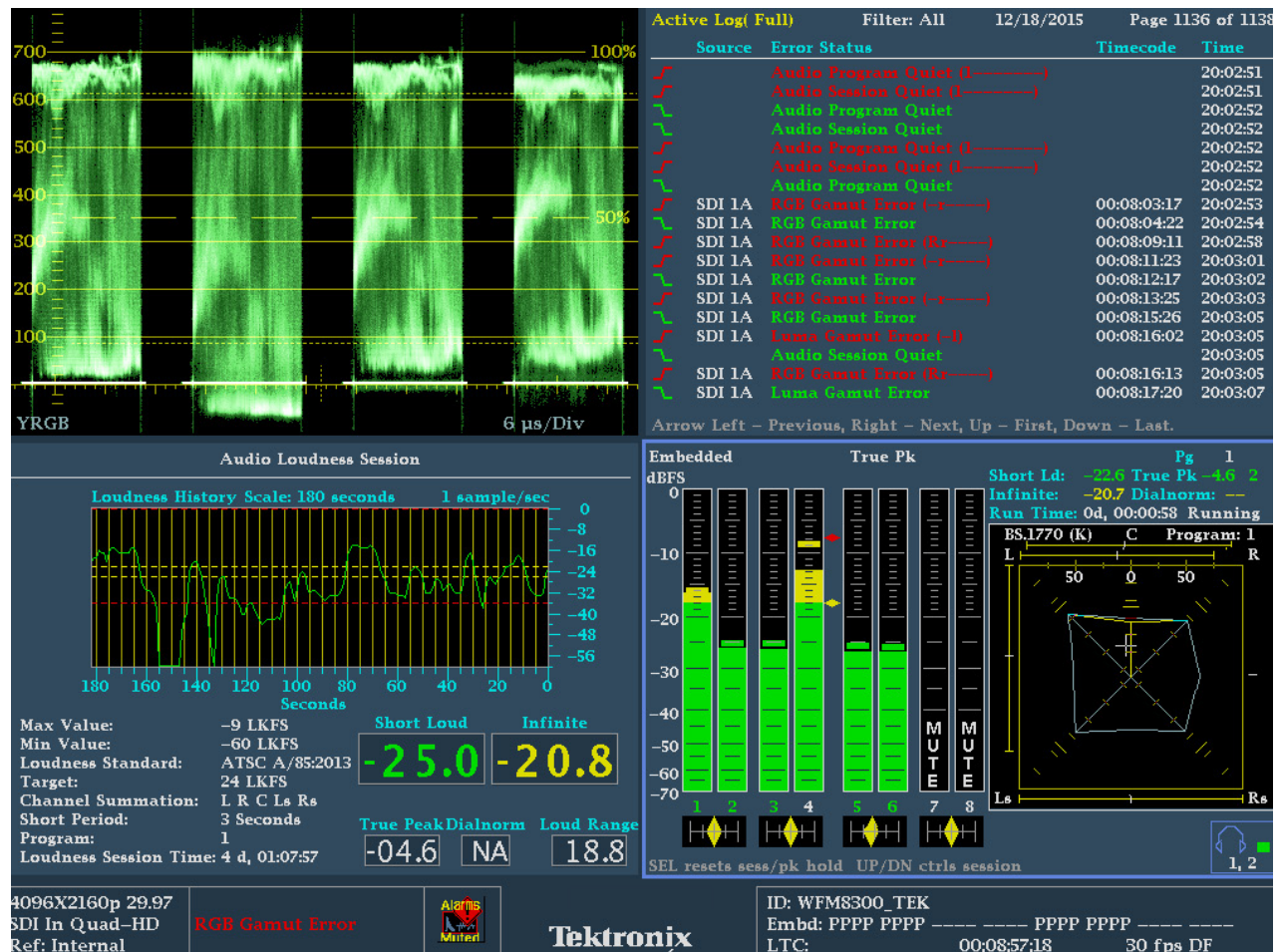
FIGURE 5-23. Four tile display showing quality assurance monitoring of video and audio with waveform, error log loudness session and audio displays.
