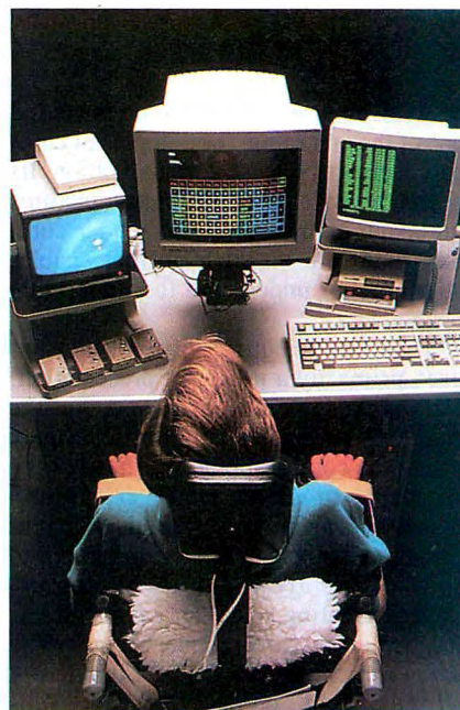
A nonintrusive eye tracker. A video camera mounted under the display tracks the position of the eye's pupil and translates the data into screen coordinates. Thus, the eyes can "point." (Photo courtesy of L. C. Technologies, Fairfax, VA)
