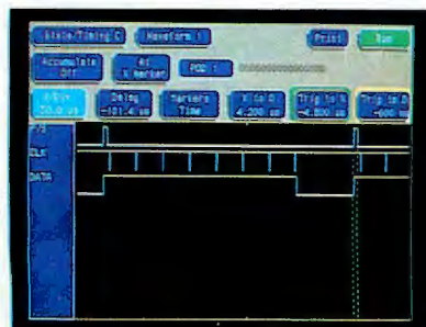
Figure C: Shown here are the timing pulses required to retrieve data from the Power Glove. P/S is the reset pulse to set the glove's shift register back to bit 0. CLK moves the register from bit to bit. After pulsing the P/S line, you sample bit 0, pulse CLK, and then sample and pulse seven more times for bits 1-7.
