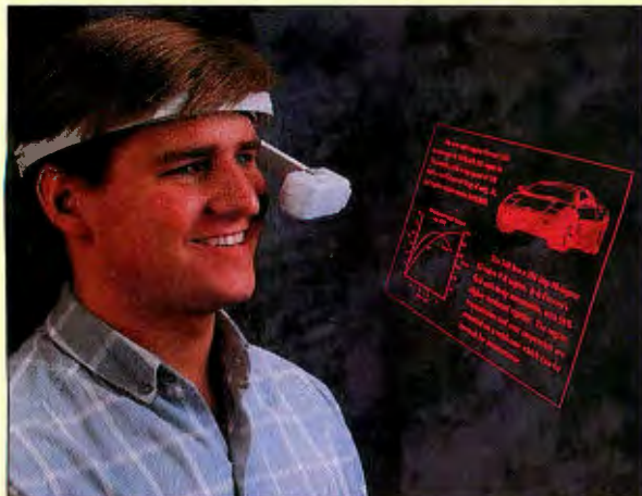
Reflection Technology's Private Eye is a virtual 12-inch CGA computer monitor with a lightweight headset.
