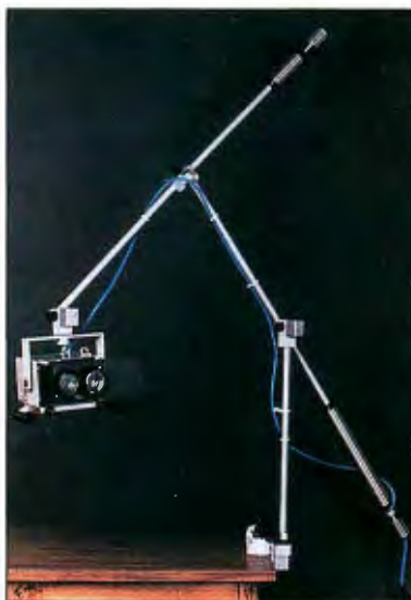
Photo B: The CCSV, a stereoscopic viewer fixed on a counterbalanced kinematic linkage, lets you easily enter and leave the virtual world.
