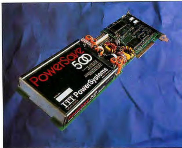
ITT PowerSystems' VIP PowerSave 500 is a backup power supply with software for saving your work and automatically shutting down your system.
