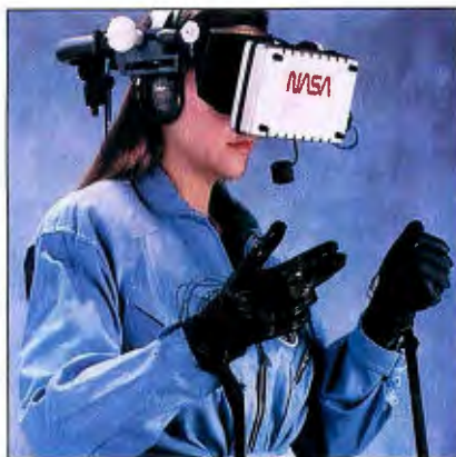
Photo 1: VIEW is a wide-angle, head-mounted, stereoscopic display system controlled by the operator's voice, position, and gestures.
