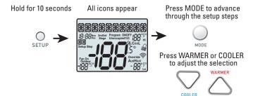
Technician Setup is for diagnostic and testing purposes and is intended for use by a qualified technician. See page 14 for more detailed instructions.
