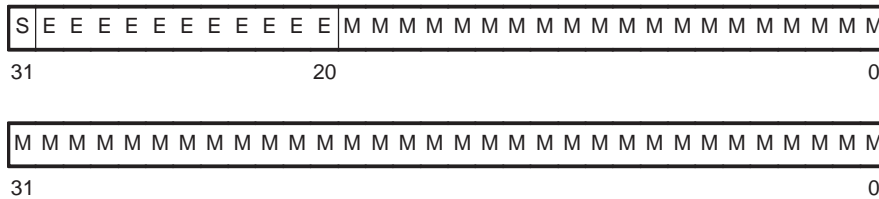
Figure 4-5. Double-Precision Floating-Point Format
