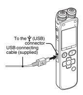
You can charge the rechargeable batteries by connecting the IC recorder to an AC outlet using a USB AC adaptor (not supplied). You can charge the batteries while you are using the IC recorder, so that it is useful when you want to record for a long time.
