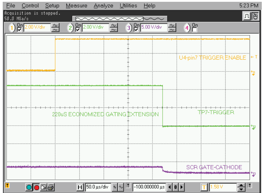
Figure 265 - Expansion of V Sense Trigger to SCR gating pulse
