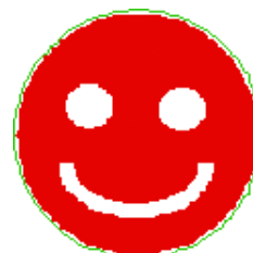
When [Extract the inside] is deactivated: A cut line will be created around the object's periphery only.
