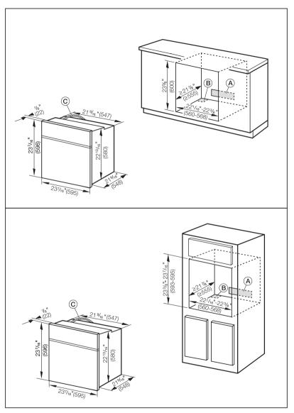
(a) Vent cut-out (min. 24"  $^2$  / 150 cm<sup>2</sup>) possible at rear of cabinet (b) Cut-out for power cord (min. 4" $^2$  / 10 cm<sup>2</sup>)
