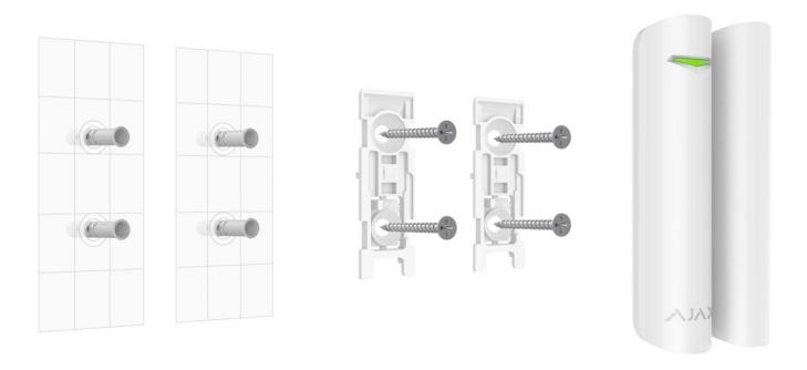
**1.** Fix the SmartBracket attachment panels and the magnet using the bundled screws. If using any other attachment hardware, make sure that they do not damage or deform the panel.
