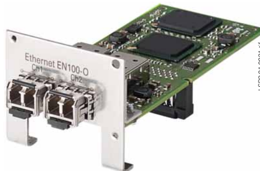
Fig. 5/89 Optical Ethernet communication module for IEC 61850 with integrated Ethernet-switch
