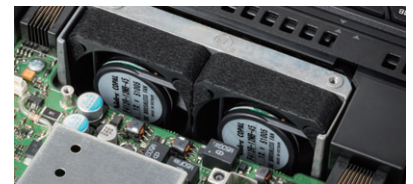
Thermostatically-controlled Dual Internal fans
