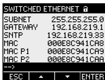
Figure 6-4 7KM PAC Switched Ethernet PROFINET expansion module settings on the 7KM PAC
