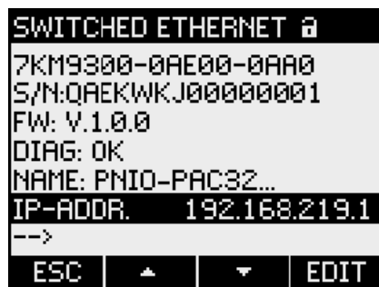
Figure 6-3 7KM PAC Switched Ethernet PROFINET expansion module information on the 7KM PAC
