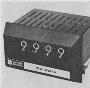
Digital panel meter series DP400 is a 10,000 count d-c voltage measuring device that provides direct digital readout of the value of the applied input voltage. Accuracy is \pm 0.02\% \pm 1 count. Three models are available with full-scale input ranges of 1, 10, or 100 v. Price (10-29) of the 100 v full scale model is $246. Computer Products, P.O. Box 23849, Ft. Lauderdale, Fla. [3611]
