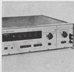
Statistical digital voltmeter designated Solartron model 1860 is for measuring and analyzing parameters of stochastic or deterministic signals. Direct digital display and analog and digital outputs of the mean, mean modulus and true rms value of the signal being analyzed, are provided. Price is $3,250; delivery, 30 days. Marconi Instruments, 111 Cedar Lane, Englewood, N.J. [3651]
