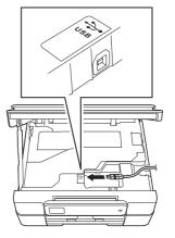
Carefully guide the USB cable into the cable channel and out the back of the machine. Connect the cable to your Macintosh.
