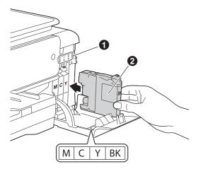
Gently push the back of the ink cartridge marked "PUSH" until the cartridge lever lifts. After all the ink cartridges are installed, close the ink cartridge cover.
