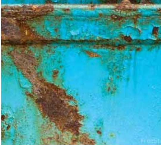
**STEEL DISPLAYS AN INCONVENIENT TENDENCY TO CONVERT INTO ITS OXIDES, THAT IS TO RUST, IN THE PRESENCE OF OXYGEN AND WATER-IN OTHER WORDS, WHEN EXPOSED TO THE AIR IT REVERTS TO THE SAME COMPOUND THAT MAKES UP ITS ORE.**
