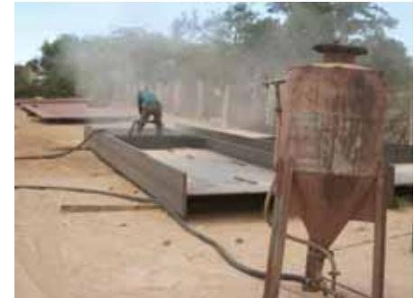
IT IS MORE TECHNICALLY ACCURATELY CALLED '**ABRASIVE BLAST CLEANING**' BECAUSE MANY DIFFERENT ABRASIVES ARE USED IN SANDBLASTING. INDEED, SAND IS NOT USED! A STREAM OF THE ABRASIVE MATERIAL IS DRIVEN FORCIBLY AGAINST THE HARD SURFACE INVOLVED.
