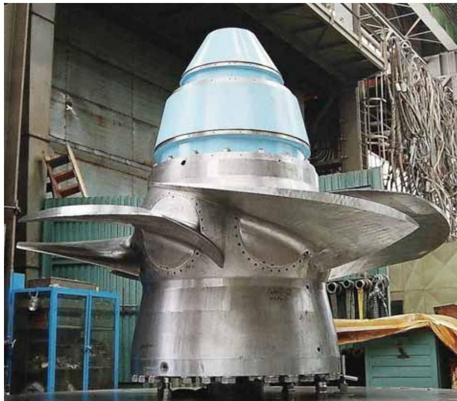
IN A KAPLAN TURBINE, COMPRESSED AIR IS USED ADDITIONALLY TO TURN THE BLADES OF THE RUNNER. AGAIN, THIS IS DONE USING PRESSURISED OIL AND HIGH-PRESSURE AIR COMPRESSORS.
