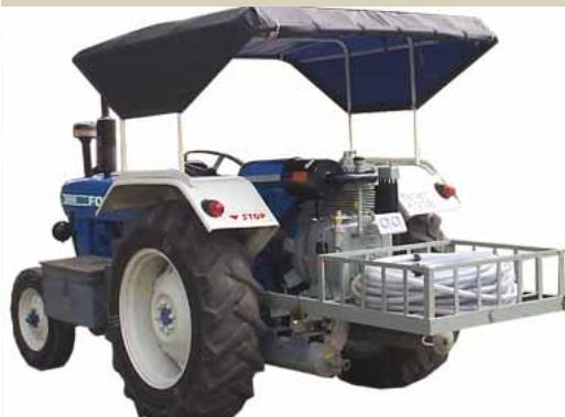
Tractor Compressors used for Jack hammer and sand blasting applications
