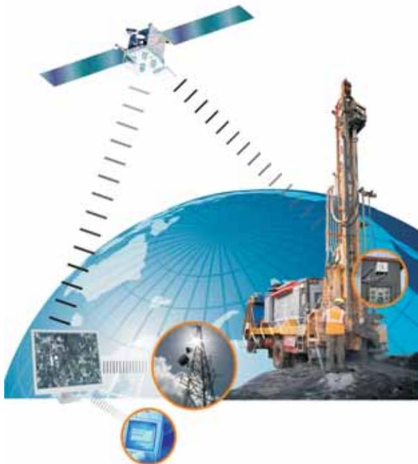
Elgi has introduced a remote monitoring system for portable air compressors in the field. The compressor tracking and remote monitoring system (CTMS) allows customers to monitor their machines in real time. It also allows them to perform preventive and corrective maintenance. Thus customers' costs of ownership are reduced, and they are provided with a wealth of information on the compressor's operation and service.
