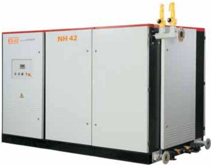
The NH-42 oil-free compressor is the latest addition to the NH series of oil-free screw compressors. These machines deliver 1800 – 2600 cfm at pressures up to 9 bar g. Reliability and low operating costs are the primary benefits that the NH series compressors offer customers. Elgi's oil-free screw compressors ensure an energy-efficient compressed air supply, thanks to the unique NH profile rotors.
