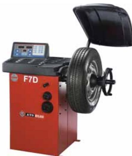
Both static and dynamic balancing can be performed using the Wheel Balancer, although the latter is the preferred type. The Wheel Balancer indicates a corrective weight of more than 100 grams for car tyres a wheel faces a run-out problem or if the cone seating is damaged.
