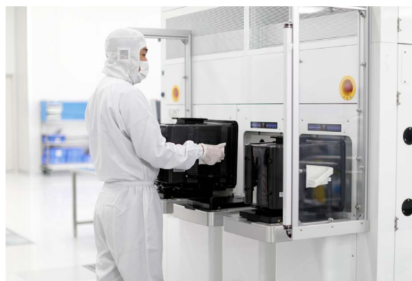
Sputtering equipment (Canon ANELVA)
