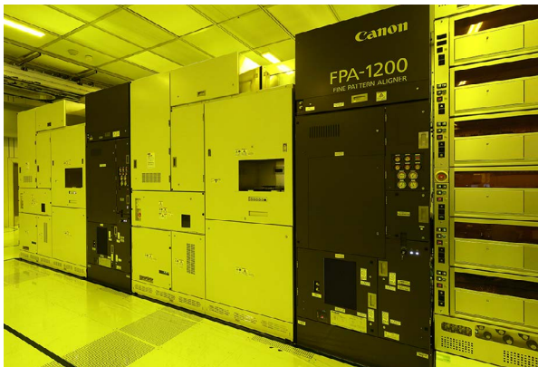
Nanoimprint semiconductor lithography equipment in testing for mass production use at a memory chip manufacturer
