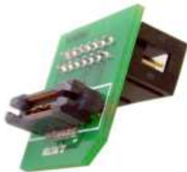
Figure 3-18: BERG14-TO-MICTOR38 Adapter (Sold Separately)
