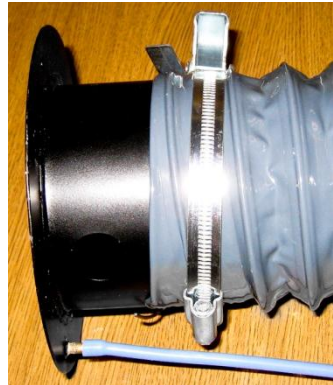
Figure 5. Connecting Pressure Tubing to Tap on Primary Duct Adapter. Bung not shown.
