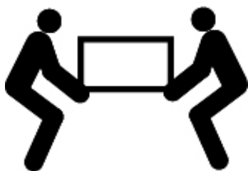
Figure 2-1. Lifting the centrifuge at both sides.
