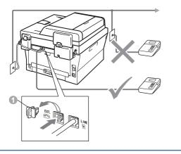
Set the receive mode to External TAD if you have an external answering machine. See Choose the correct Receive Mode on page 8. For additional details, see Connecting an external TAD (telephone answering device) in the Basic User's Guide.
