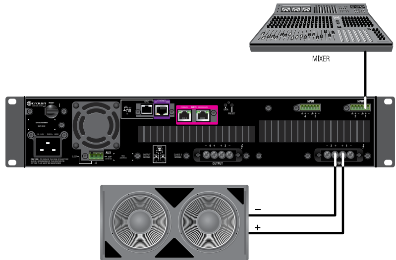
Figure 23: System wiring in Bridge Mono mode
