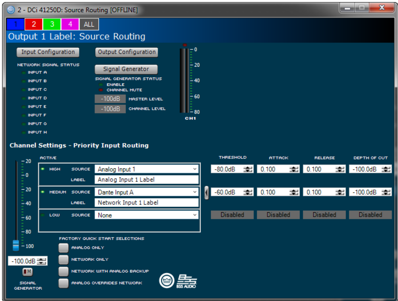
Figure 41: Advanced Source Routing panel
