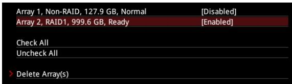
3. Select the desired array and change the setting to **Enabled**.
