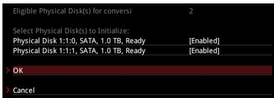
3. Select desired disks by changing the Physical Disk setting to **Enabled**.
