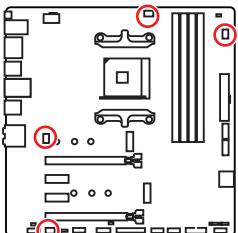
Automatically detect mode fan connector
