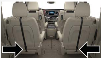
Rear Seat Tether Strap Attachment (Second Row 7 Passenger Stow n' Go Anchorage Shown)
