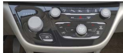
Automatic Climate Controls On The Faceplate
