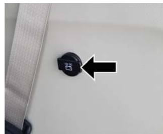
Rear Power Outlet
