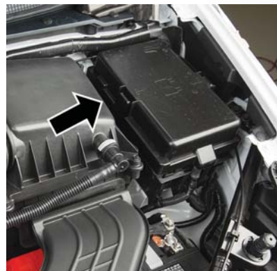
Power Distribution Center
