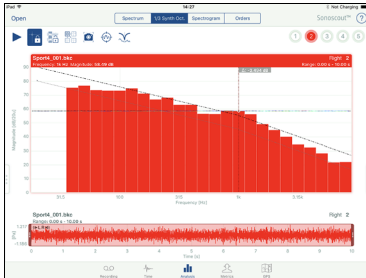
Fig. 8 Target curves can also be used as tolerance bands – the dark grey curve is set to +2.5 dB, the light grey to -2.5 dB. The \Delta cursor (highlighted) indicates the difference between the upper target and the measured spectrum
