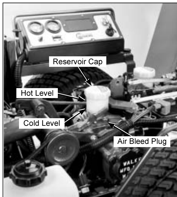
Transmission Reservoir and Air Bleed Plug Location
