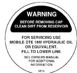
Hydrostat Oil Reservoir (5810)
