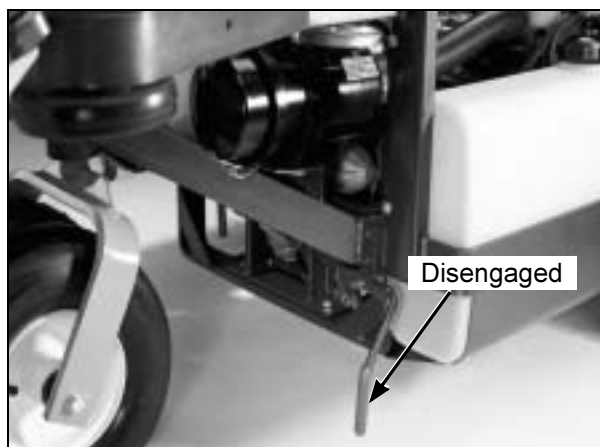
Jackshaft Drive Belt Release
