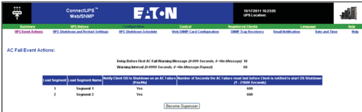
Figure 182. UPS Shutdown and Restart Settings
