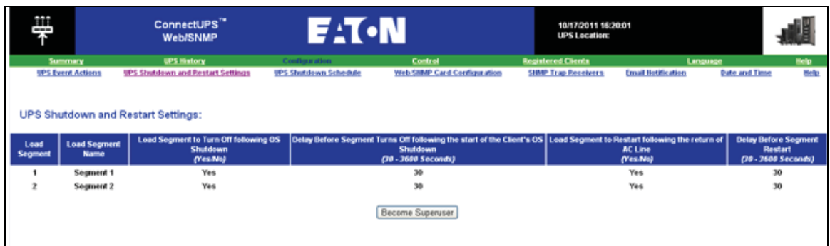
Figure 179. UPS Shutdown and Restart Settings
