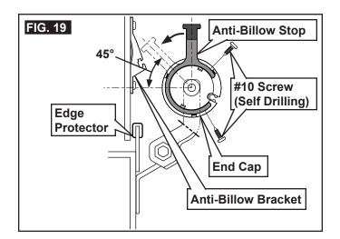
Determine required configuration of anti-billow bracket and spacer (spacing from RV wall) to ensure anti-billow stop will **NOT** rotate past a 45° angle (toward RV wall). See (FIG. 19) & (FIG. 20).
