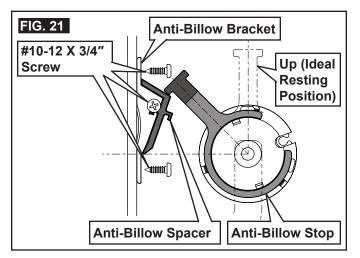
5. Place and tighten #10 self drilling screws (provided) through anti-billow stop and into end cap. See (FIG. 18) & (FIG. 19).
