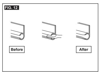
5. **NOTICE** Do **NOT** unfurl more than 1 revolution of fabric, as this could cause issues with awning [closing / opening] correctly.
