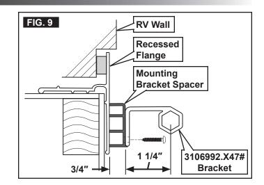
b. With mounting bracket aligned correctly, slide onto extension (attached to LH arm), and tape in place.
