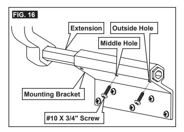
8. Place and tighten #10 X 3/4" screws (provided) through middle and outside holes of mounting bracket and into extension. See (FIG. 16).
