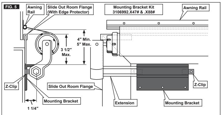
Determine mounting bracket location relating to awning rail and slide out room flange. See (FIG. 3), (FIG. 4), (FIG. 5), (FIG. 6), & (FIG. 7).
