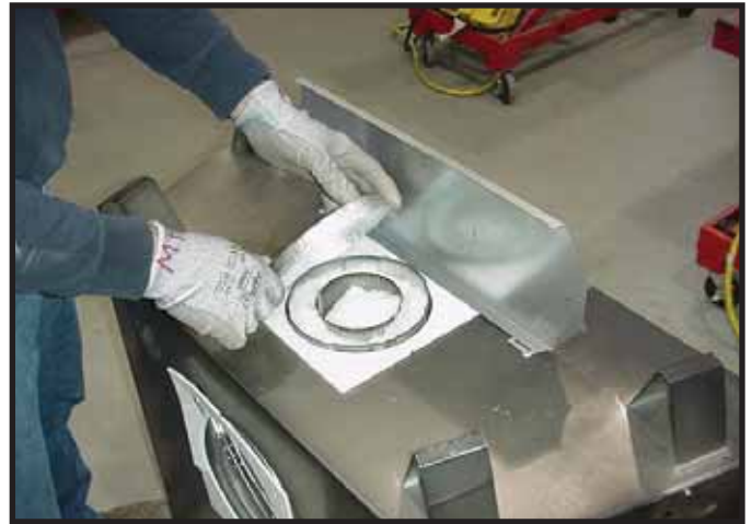
Figure 9.4 Remove the seal cap.
