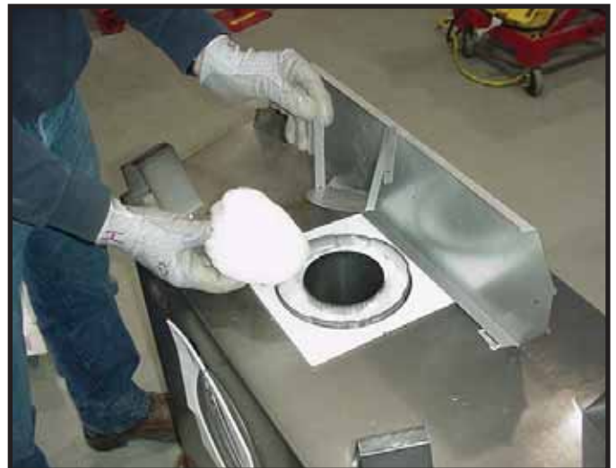
Figure 9.5 Remove the insulation basket and white insulation from the center vent pipe.
