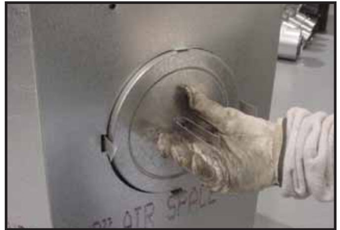
Figure 9.10 Fold the center parts of the retaining band out and use to remove the seal cap.
