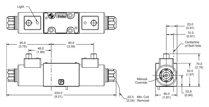
Note: 22.0 mm (0.87") from bottom of bolt hole counterbore to bottom of valve.
