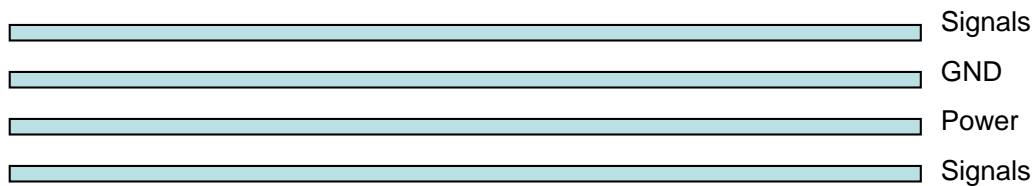
Figure 15: Typical 4-layer PCB construction
