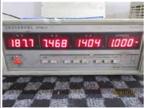
Low voltage start check
