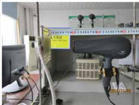
Outlet temperature check
