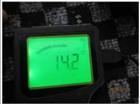
Air flow speed check
