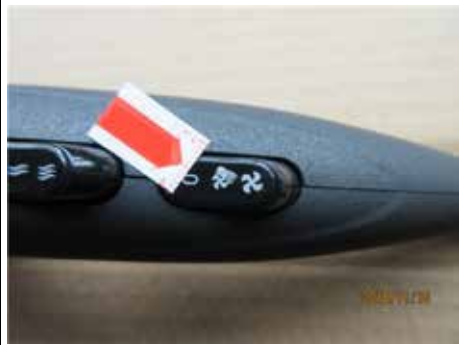
Residual sticker on the switch
