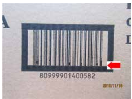
Remark 4, Slight poor printed mark was found on the one side of the carton barcode
