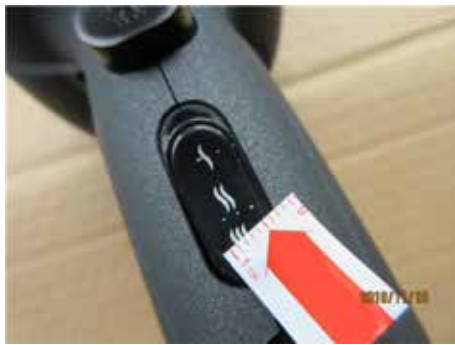
Poor silk-screen on the switch
