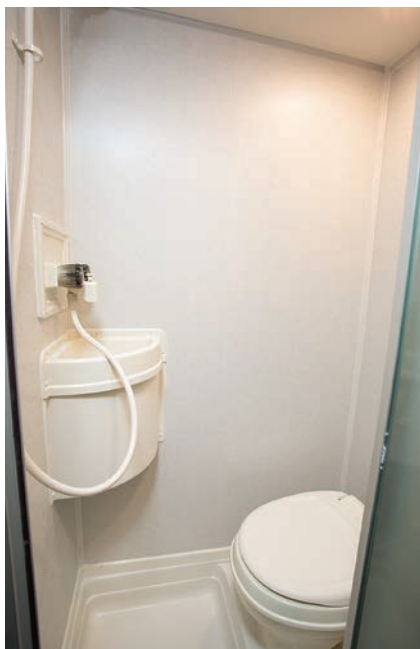
The wet bath has a sunken shower pan and a raised toilet platform, plus a separate sink faucet in addition to the showerhead.
