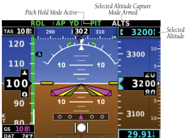
Figure 3-8 Pitch Hold & Selected Altitude Capture Modes
