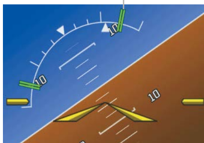
Figure 3-27 Roll Increasing to ESP Engagement
