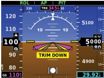
Figure 3-22 TRIM DOWN Alert
