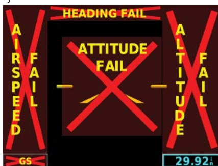
Figure 1-2 G5 PFD Page Failure Annunciations
