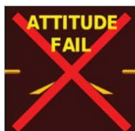
Figure 1-6 Attitude Failure Indication
