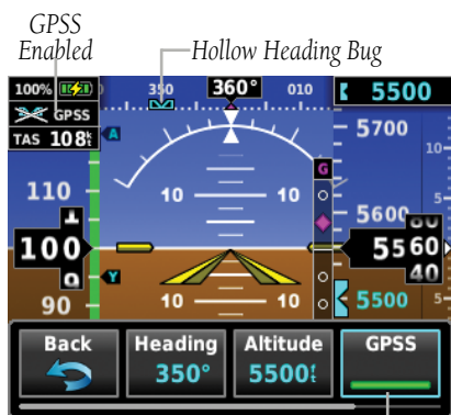
Figure 4-3 GPSS Enabled - PFD
