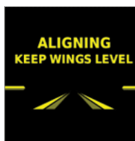
Figure 1-5 Attitude Aligning Keep Wings Level Indication
