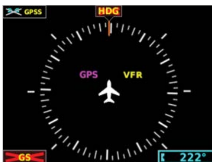
Figure 1-3 G5 HSI Page Failure Annunciations
