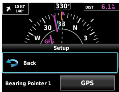
Figure 2-20 Bearing Pointer Setting
