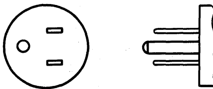
Figure D-3. Plug with Earthing (Ground) Pin – 15-A Max, 125V (Canada and U.S.A.)
