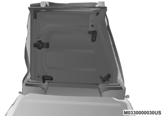
Left Panel — Latches Facing Upward
