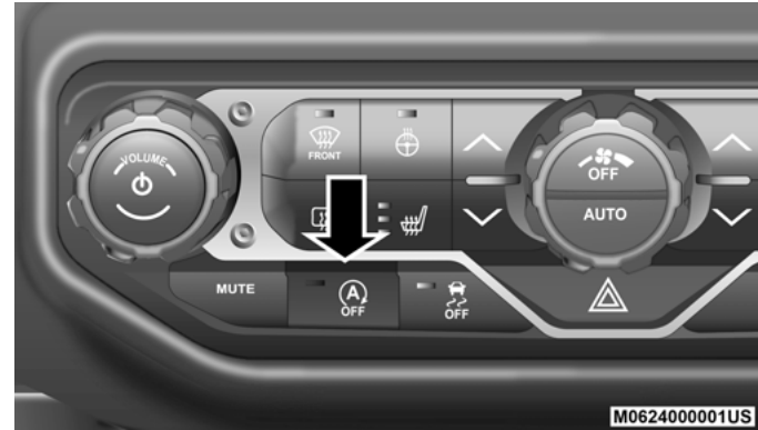
Stop/Start OFF Switch
