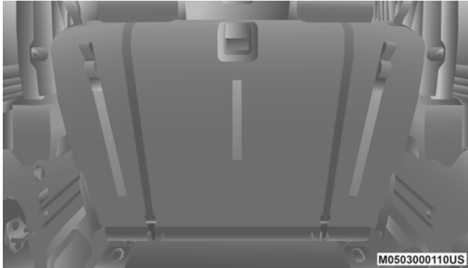
Tether Strap Mounting (Two-Door Models)
