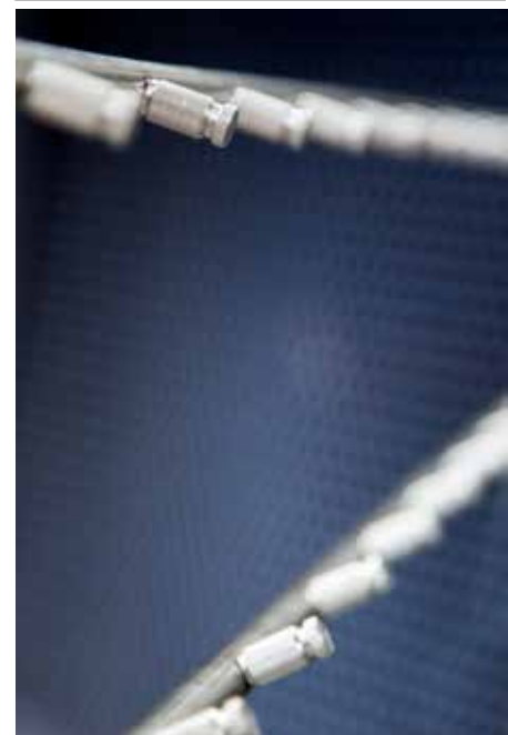
FIGURE 46-2: TOP HALF OF MANIFOLDS ANGLE DOWNWARDS, OTHER HALF ANGLE UPWARDS
