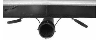
Black/Grey Tank Drain and Valves
