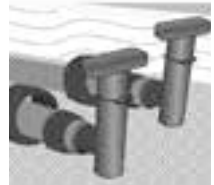
Low Point Drains
