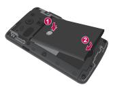
3 Align the back cover over the battery compartment 1 and press down along the outer edges of the back cover 2.
