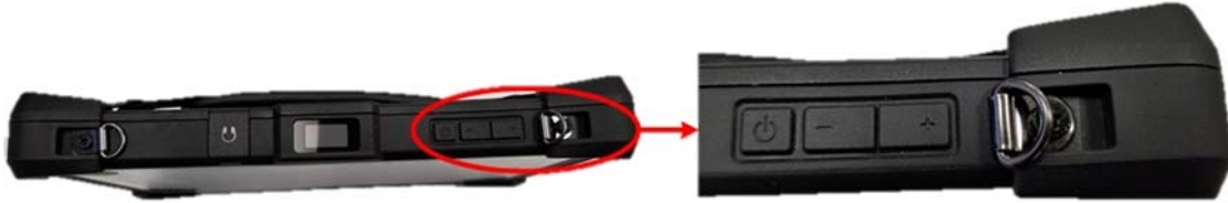
Figure 6. Press + Button To Unlock The Tablet
