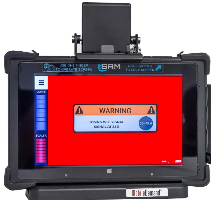
Figure 10. Wi-Fi Signal Strength Warning Example
