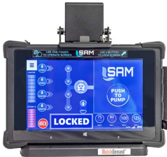
Figure 2. Emergency IDLE Activation (From A Locked Screen)
