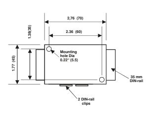
REAR PANEL MOUNTING DIN RAIL OR 2 SCREW
