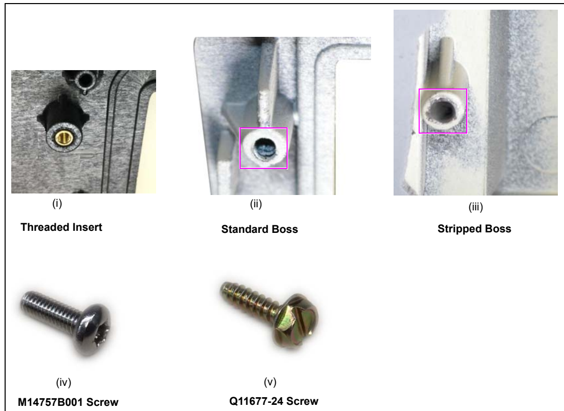
Figure 2: Examples of Threaded Insert, Standard, and Stripped Bosses
