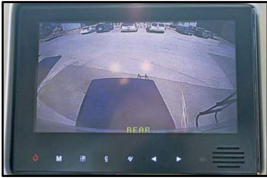
Figure 16-1: Rear View Camera Monitor System
