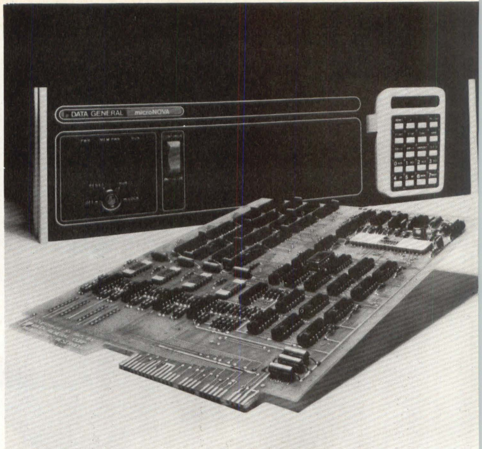
Fig 4 Data General microNOVA 16-bit computer, available in board or cabinet configuration, uses mN601 CPU chip, can provide up to 315 K word memory with optional dual diskette.
