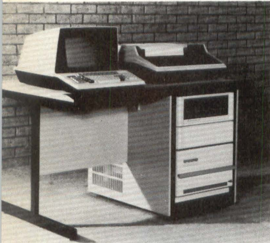
Fig 3 Texas Instruments model 990/4 16-bit microcomputer, based on TMS 9900 microprocessor, with 24K x 16 words of memory, floppy-disk ROM loader, video terminal and floppy disk, can be programmed in several high-level languages such as FORTRAN IV, COBOL and Multiuser BASIC.
