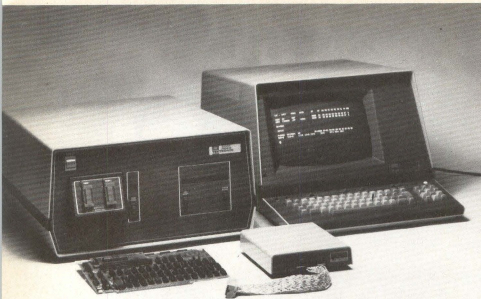
Fig 6 Electronic Tool Company ETC-1000 microcomputer, based on 8-bit 6502 microprocessor, available in several configurations, can have up to 32 K of RAM and dual floppy disks.
