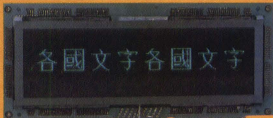
Vacuum Fluorescent Module, super fast bit mapped display. 256 x 64 pixels.
