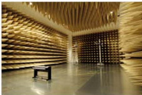
Radio wave darkroom used for electromagnetic wave measurement
