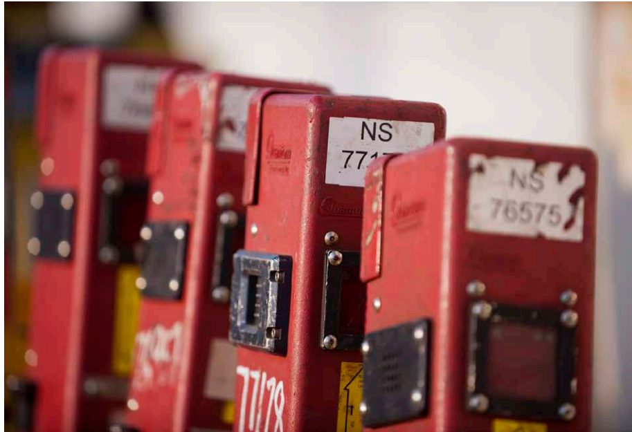
■ Pictured here are end-of-train devices, used to monitor a train’s brake line pressure.
