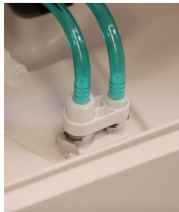
Figure 33: HPM Gas Lines Connections
