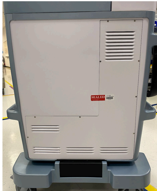
Figure 24: Photograph of Tamper Evident Seal on Console
